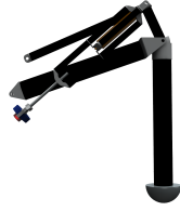
Fig. 15. Skeldar V-200 leg assembly with custom electric actuation
