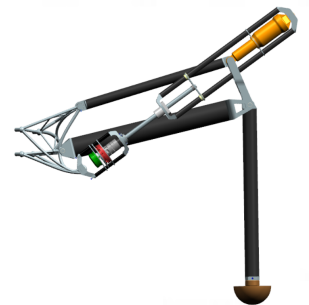
Fig. 3. Leg structure including the actuation, rods black, joints and spindle grey, brake red, damper yellow, motor green, foot brown
