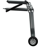
Fig. 17. AS332 Super Puma leg assembly with wheel and hydraulic actuation
